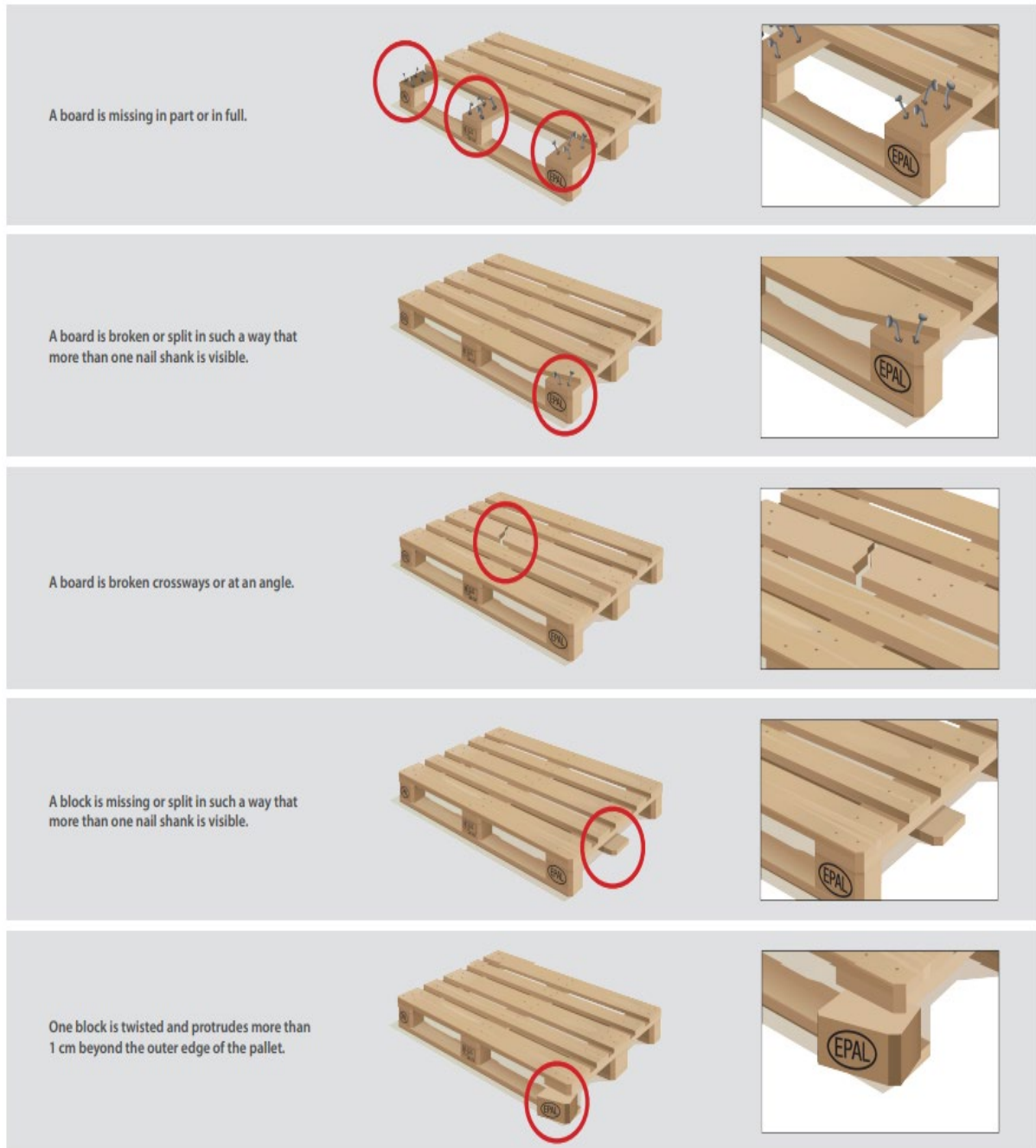
Picture 1: Not accepted pallet quality, source EPAL Quality and Exchange GB.pdf (epal-pallets.org)
